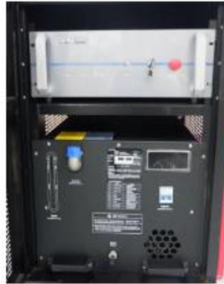
Laser source and water chiller, compact size
