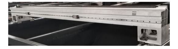
Better performance and looks brighter than cast aluminium, stable and not easy deformed, light in weight and good in dynamic performance. After secondary vibration and aging treatment, it is finished to ensure the strength, rigidity and stability of the beam.
