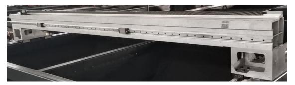
Better performance and looks brighter than cast aluminium, stable and not easy deformed, light in weight and good in dynamic performance. After secondary vibration and aging treatment, it is finished to ensure the strength, rigidity and stability of the beam.
