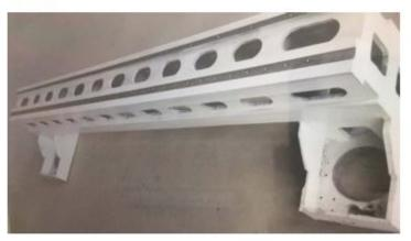
The whole beam is made of aluminum alloy material, which is light in weight and good in dynamic performance. It adopts integral casting method, and is roughened after annealing to eliminate internal stress. After secondary vibration and aging treatment, it is finished to ensure the strength, rigidity and stability of the beam.
